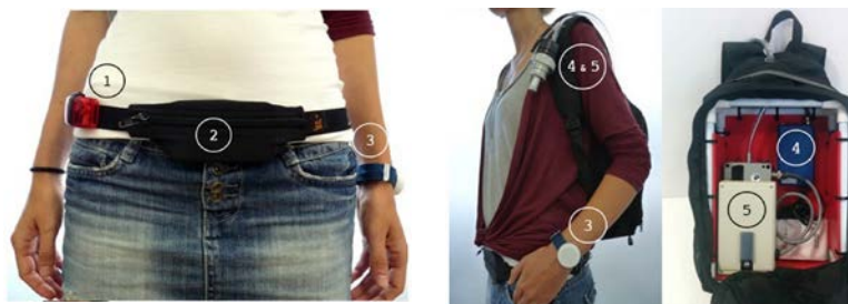
Figure 8: Measurement kit used in the HELIX project to characterise individual exposure (Donaire-Gonzalez et al. , 2019)
